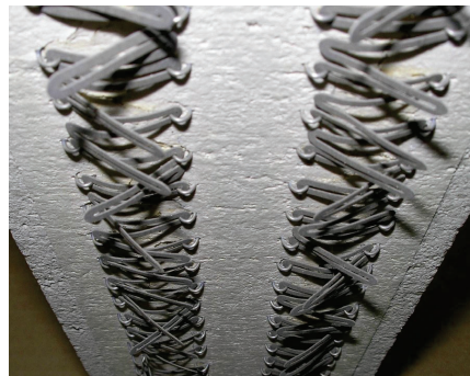
Pinned elements after high temperature cycling
