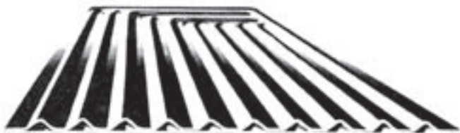
Fig. 2-2 In single embossed PLATECOIL, one sheet is not embossed, thus providing a flat surface and a reduction in PLATECOIL thickness of about one half.
