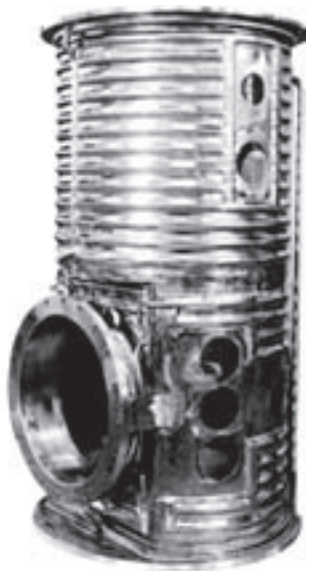
Completed shroud assemblies as fabricated and tested with all cryogenic special features described in the typical specification above.
