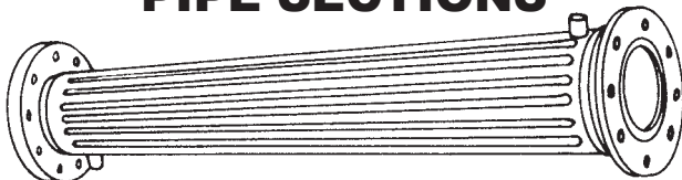
Fig. 36-3 PLATECOIL Jacketed Pipe
