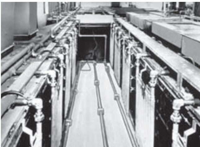
Fig. 57-1 Type 316L stainless steel full solution annealed PLATECOIL for cooling sulphuric acid anodizing solutions. They also act as cathode area.
