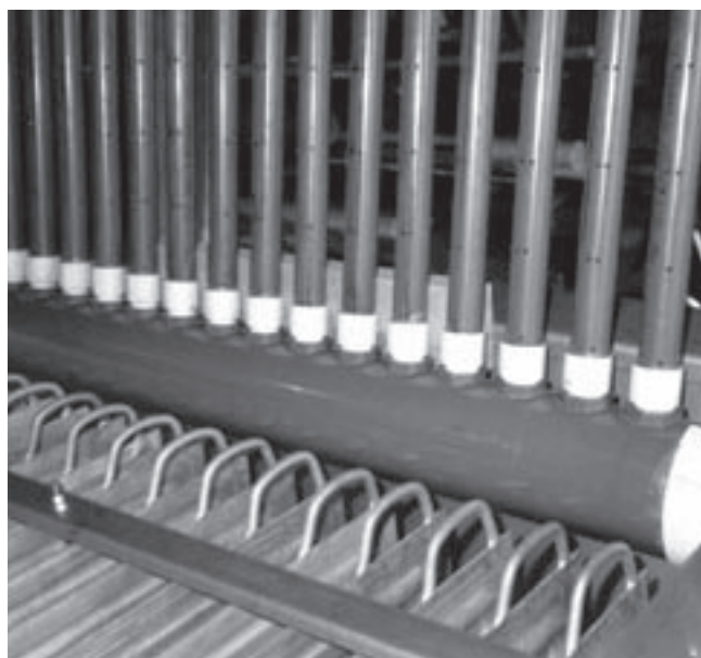
Fig. 56-2 These are Style 50D Serpentine PLATECOIL in a falling film chiller for a special anodizing operation.
