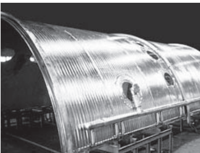
Completed shroud assemblies as fabricated and tested with all cryogenic special features described in the typical specification above.
