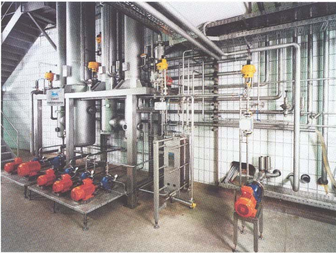
Bottom of the stripping column, condenser and heat exchanger from SIGMATEC
