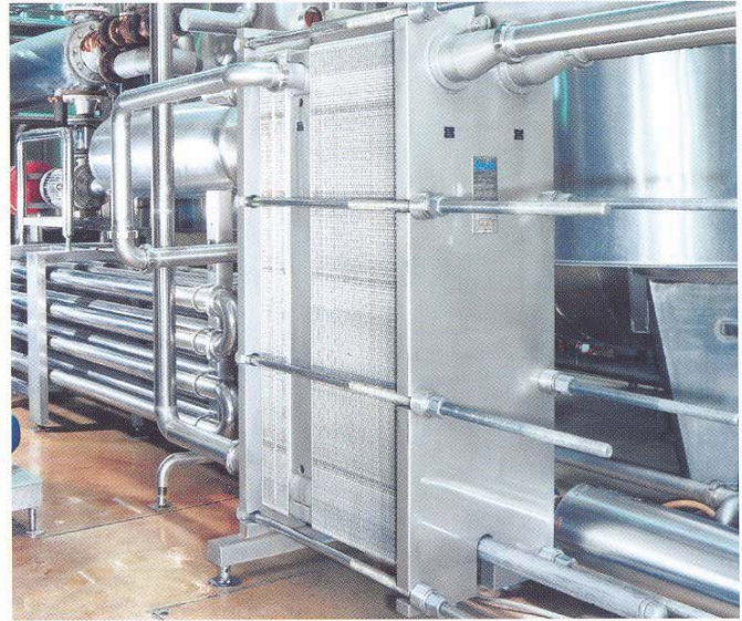
SIGMATHERM Short-time-heating system with SIGMA 65 for 300 hl/h wheat beer
