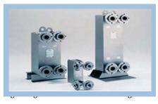
Fully welded and require no gaskets. Available in all 316SS construction, titanium and other higher alloy materials. These units have a design temperature of 750°F and can handle operating pressures as high as 360 psi with an ASME Code stamp.
