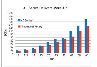
AC Series offers you the next level of sophistication. Featuring industry leading CFM performance, quiet {as low as 67 dB(A)} operation, electronic controllers, energy saving soft-start Wye-Delta motor starters, TEFC motors, air-cooled aftercoolers and optional integrated refrigerated air dryers.
