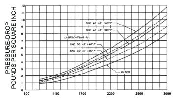
FLOW IN U.S. GALLONS PER MINUTE Recommended pressure drop is 2 to 7 psi.
