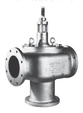
AMOT Model D Thermostatic Valves are fully automatic, 3-way fluid temperature controllers for diverting applications. They are used to provide reliable control lubrication oil cooling systems. These valves are suitable for process control and industrial applications where fluids must be diverted depending on their temperatures. They may also be applied to cogeneration systems to control temperatures in the heat recovery loop assuring proper engine cooling and maximizing heat recovery.
