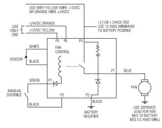
NOTE: This switch should be fused to prevent damage if ground is lost. A 30 amp fuse is required in the power supply.
