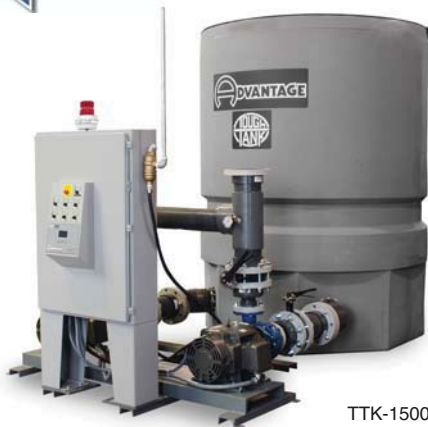
TTK-1500 pump tank station with polyethylene reservoir and 3 pump system shown with Checkmate™ monitoring and system control instrument
