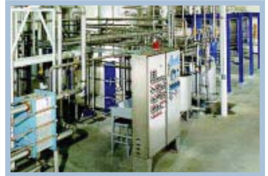
A five-effect SIGMASTAR® Plate Evaporator installation.
