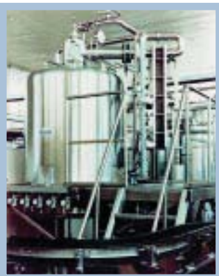
Mash heater for high viscosity fruit pulp.
