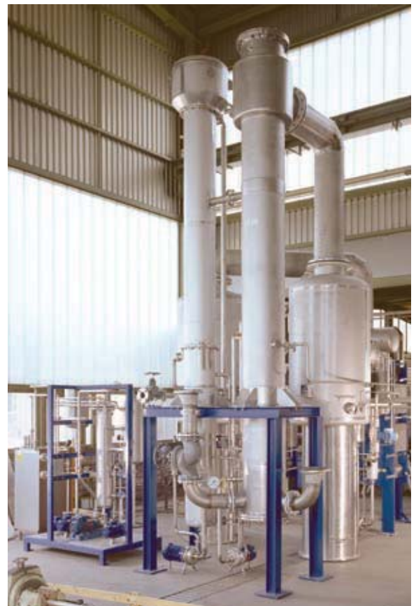
Evaporator with an Aroma Recovery System
