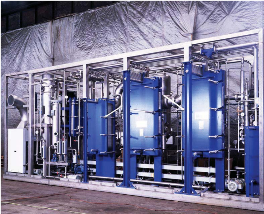
Rear view of API Schmidt-Bretten pilot plant showing left to right: a refrigeration system, an aroma recovery unit, a model Sigma 48 plate condenser and model Sigma Star 90 1st and 2nd effect plate evaporators.
