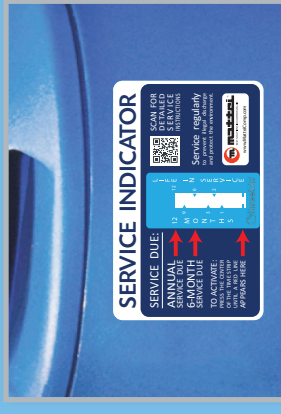
Figure 2: MCS Service Indicator ensures timely replacement of media
