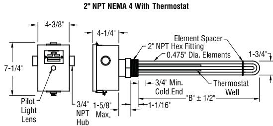
**Single-Pole, Single-Throw Thermostat on 1-1/2", 2" and 2-1/2" Pipe Thread Heaters** - Where single-pole control for pilot duty is adequate, and neither pilot light nor an ON/OFF switch is required. 0°–100° F and 60°–250° F temperature ranges are available.
