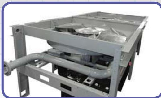
Two 72" diameter, 8-blade, high output fans are stationed beneath the radiator stack, pushing 148,000 CFM of air through the copper cooling fins when operating at full speed.
