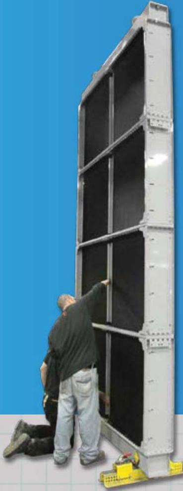
A Polar Pod unit contains 16 individual 11.5 sq. ft high efficiency radiators...eight dedicated to the jacket water cycle, the other eight to the aftercooler.
