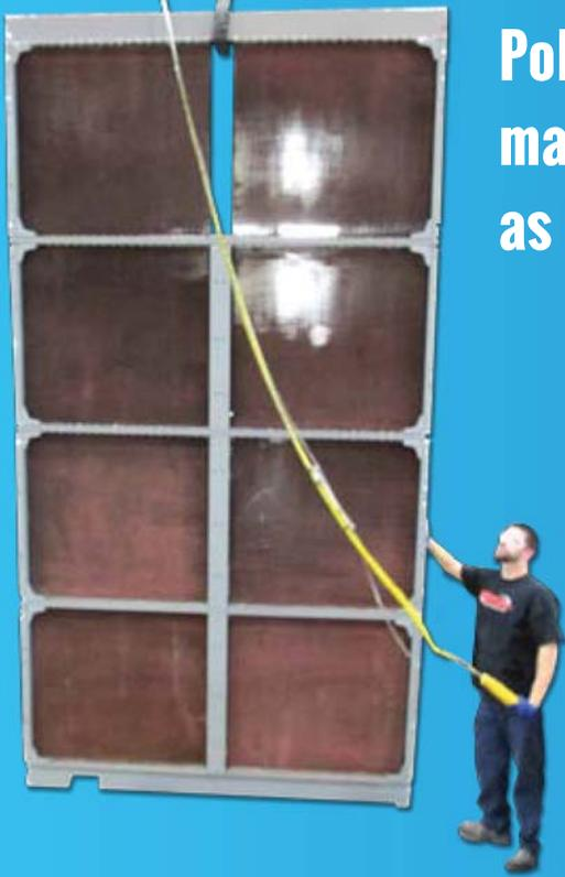
A Polar Pod unit contains 16 individual 11.5 sq. ft high efficiency radiators...eight dedicated to the jacket water cycle, the other eight to the aftercooler.
