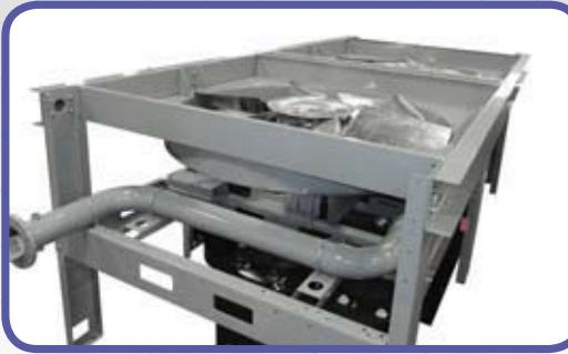
Two 72" diameter, 8-blade, high output fans are stationed beneath the radiator stack, pushing 148,000 CFM of air through the copper cooling fins when operating at full speed.
