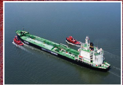
Asphalt Commander. Three Heatec vertical heaters, directly behind the pilot house, maintain the tanker's cargo of 8 million gallons of liquid asphalt at 280 degrees F. Heatec designed, built and installed the heaters when the ship was converted from a U.S. Navy fuel tanker. The heaters provide 15 million Btu/hour each and heat thermal fluid circulating through 22 miles of piping in 14 compartments
