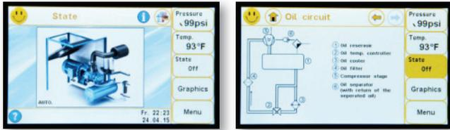
Continuously tracks pressure, temperature, air quantity and usage to easily diagnose and optimize your plant's air system.
