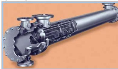
Straight-tube, removable bundle exchangers made from standard components. Floating tube sheet for seal leak detection and easy maintenance. Diameters from 3" (7.6 cm) to 42" (106.68 cm). ASME, API, TEMA, ABS and other codes available.
