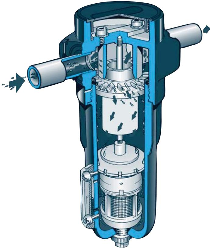
**Aftercoolers and Moisture Separators** work hand-in-hand to cool and remove damaging water from compressed air systems.
