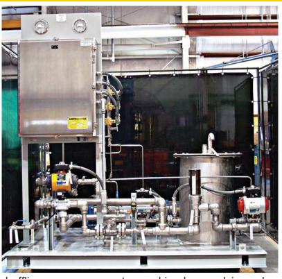
All 3 systems are designed to perform online and offline compressor water washing by supplying mineralized water or water and detergent to the gas turbines spray nozzles internal to the compressor plenum. Online compressor washing is utilized to prevent build up of heavy deposits on the compressor blades. Offline compressor washing is preformed to eliminate heavier, more difficult accumulation.
