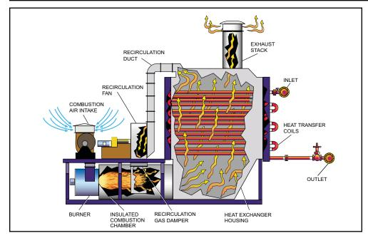
The product is heated as it flows through the heat transfer coils. The coils are heated by convection gases as they pass around the outer surfaces of the coils. The gases are recirculated to boost efficiency and to limit radiation from the burner flame.
