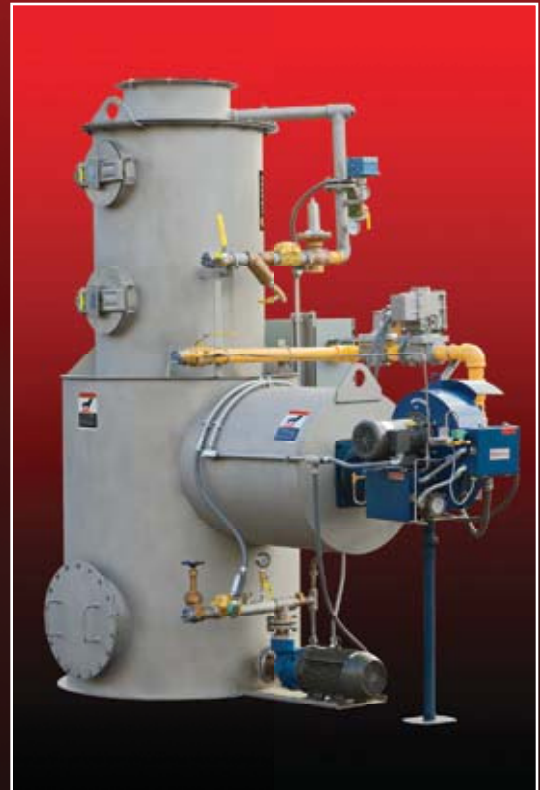
Hatches on the heater's upper section provide full access to the spray nozzle and packing area for inspection & maintenance. A manway on the lower section allows internal access to the combustion area.
