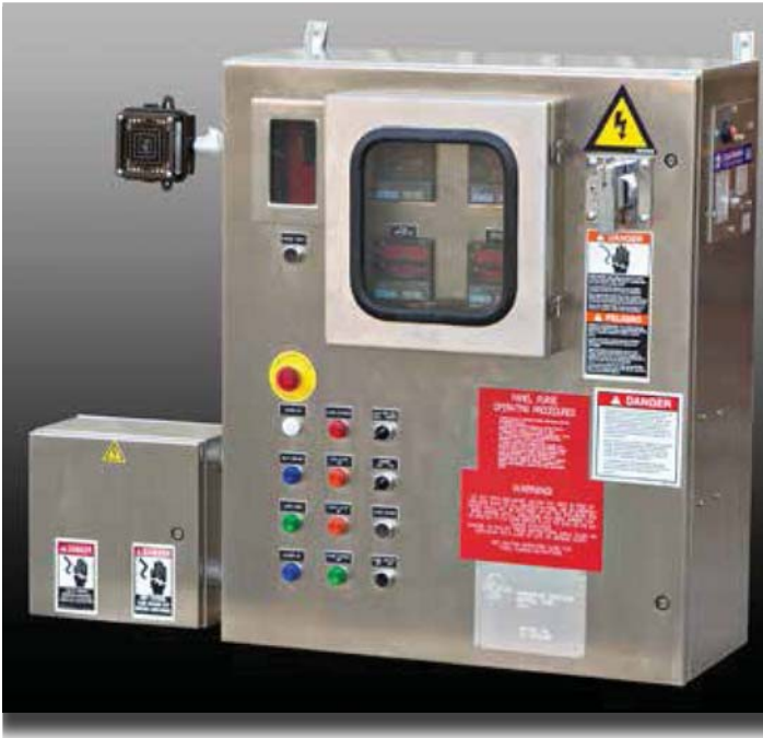
A typical NEMA Type 4 panel for areas temporarily exposed to combustible gases. Panel is equipped for Type Z pressurization and also purges the small panel on the left.
