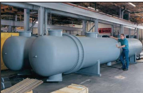
TEMA BEU Exchanger for Wastewater Treatment
