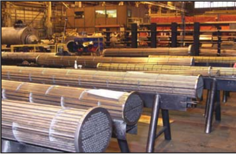
API Basco Shop Bundle Assembly Area
